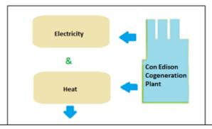
Our combined-heat-and-power cogeneration plants are about 60% efficient, compared to that of a conventional plant at 50%. A LEED guideline considers this cogen electricity as an energy cost credit when energy modeling, which grants the building project LEED points.
